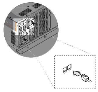
Figure 8 Connecting the BTS Cable to BTS Jack
